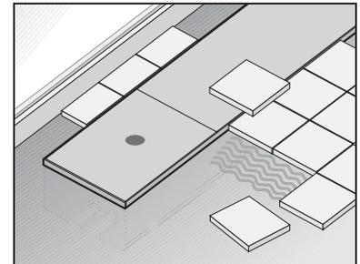
Adjustment blocks serve for the alignment of the system convectors and for protecting against suspension during the floor pavement installation.
